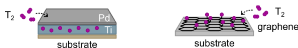
Figure 1: Schematic of tritium loading in metal samples (left) and on graphene (right).
