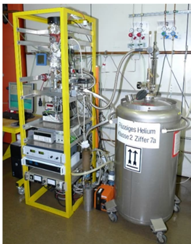
Figure 1: First low-temperature thermal desorption spectroscopy (TDS) experimental set-up with liquid He cooling at Max Planck Institute in Stuttgart.
